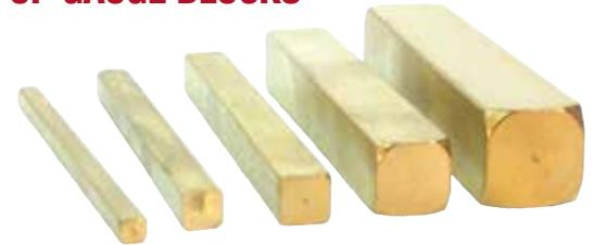
Our Square Gauge Blocks are a quick way to make many easy, accurate set-ups. A great way to make exact depth movements on plunge routers. On table routers, they're perfect for setting distances from the fence to the cutter, or for checking the bit height above the table. Supplied in 1/8", 3/16", 1/4", 3/8", and 1/2" squares. Blocks can be "stacked" to cover a wider range of sizes. A very helpful tool!
