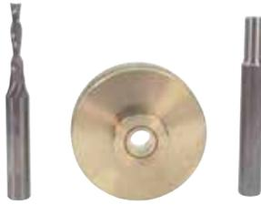
Whiteside's Brass Inlay Kits allow you to make perfect fitting inlays for decoration or repairs. Simply cut your template from 1/4" thick material and trace it with your router to cut both the cavity in your workpiece and the matching inlay to be inserted. Instructions are included. Our kit includes a special centering pin to insure exact alignment with router spindle. Each kit includes a Solid Carbide Down-Cut Spiral router bit.
