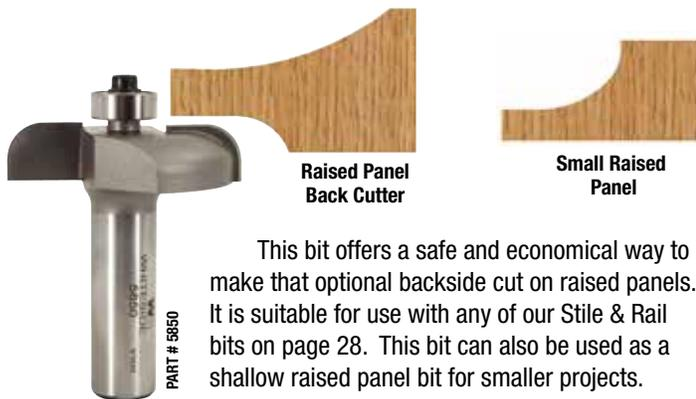
This bit offers a safe and economical way to make that optional backside cut on raised panels. It is suitable for use with any of our Stile & Rail bits on page 28. This bit can also be used as a shallow raised panel bit for smaller projects.
