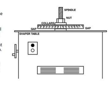
REMEMBER: For a proper fit, your shaper must be aligned. Before using any shaper cutter, always check your spindle to ensure it is square with the shaper table. Misalignment here causes off pattern and fitting problems.
