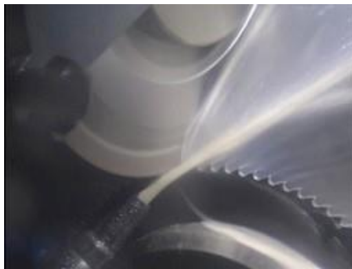
HSS circular saw grinding by CBN wheel
