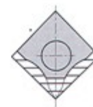
Insert blank is 12x12mm Profilable Area (lines) Scale 1:1
