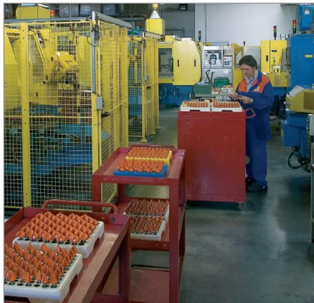
*Loading the automated multi-axis CNC sharpening machines.*
