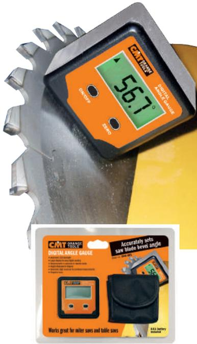
The digital angle gauge is a mini waterproof digital protractor that provides digital readings between  $\pm 90^\circ \times 4$  with a resolution of  $0.1^\circ$  and features auto shut off after 5 minutes. It is small enough to be carried around in your pocket and the LCD screen is easy to read. It incorporates magnets in the base for adhesion to any ferrous surface to accurately measure miter and bevel angles on miter saws, saw benches, etc.
