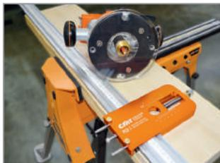
Prepare your router: Install the guide bushing rings into the bore baseplate and then attach it as the base for your router. Select and insert your router bit. Prepare the Adjustable Guide Rail & Straight Edge Clamp: Position both the adjustable straight edge clamp and then the adjustable precision router dado jig onto your workpiece. Then using the adjustable thumb screws, secure it. Once assembled, ensure that the adjustable precision dado jig slides freely.
