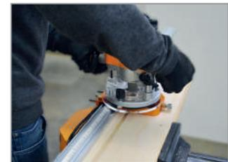
Holding onto your router in position, power on and begin making the cut by pushing forward and back on the straight edge clamp using the precision router dado jig as a guide. Makes impeccable grooves and dadoes along the length of your workpiece.
