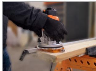
Insert your router into the center hole of the adjustable precision router dado jig.
