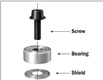
**Caution:** be sure to keep the black washer right side up to correspond with the bearing rotation during reassembly.
