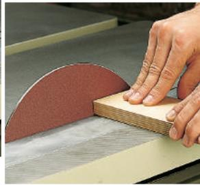
Before starting a new project, balance your CMT blade in your table saw with the CMT calibration & sanding disk. Mount your calibration & sanding disk in your table saw and line it up with a square for accuracy. Remove the calibration and sanding disk and mount your saw blade for clean, accurate cuts. You can even use the calibration and balance disk as a sander by attaching self-stick sandpaper and installing the disk in your table saw.
