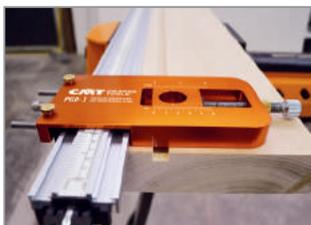
For creating dadoes that exceed router width, using the adjustable gauge, simply select the desired width on the graduated scale.
