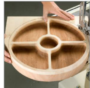
Bandsaw the exterior to final shape.
