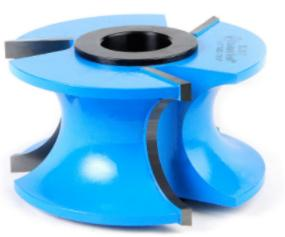
Item #SC572, Amana Tool Carbide-Tipped 3-Wing Bullnose 3/4" Radius x 1-1/2" in Bead Radius x 3-13/16" Dia x 1-5/8" x 1 & 1-1/4 inch Bore \$195.09
