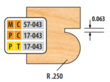
Item #PC 17-043, Freeborn Bead Cutter - 1-1/4" Bore (Pro-Line), 3-Wing, 4" Dia, .250 Bead Radius \$236.30
