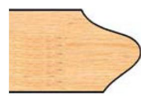
Item #PC 17-001, Freeborn Door Edge Detail Shaper Cutter - 1-1/4" Bore (Pro-Line), 3-Wing, 4" Dia, 1" Tip \$277.10
