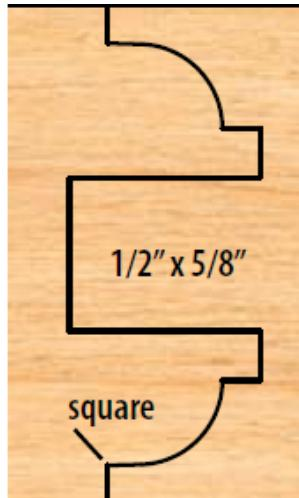
**Item #PC 11-041, Freeborn (8-Piece Cutter Set) Double Sided Cope and Pattern - 1-1/4" Bore (Pro-Line), 4" Dia, 3-Wing**
