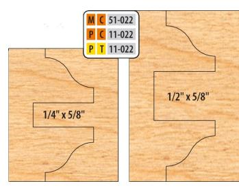
Item #PC 11-022, Freeborn (8-Piece Cutter Sets) Double Sided Cope and Pattern - 1-1/4" Bore (Pro-Line), 4" Dia, 3-Wing \$1,190.00
