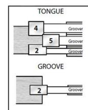
Each function of the 6 piece cope & pattern set requires a different cutter configuration. For desired results, use the following guide to set up each operation.
