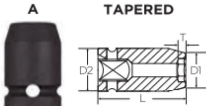
**Item #MSP27162, Vega 6-pt Fixed & Spring-Loaded Magnetic Impact Sockets Long Length - 3/8" Sq Drive (SAE)**
