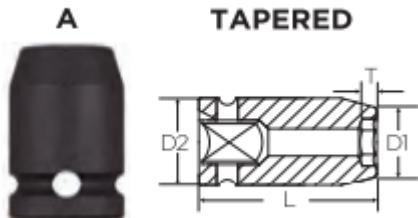
**Item #MSP20382, Vega 6-pt Fixed & Spring-Loaded Magnetic Impact Sockets Long Length - 3/8" Sq Drive (SAE)**
