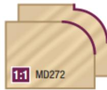
A second shoulder can be produced with the 3/8" bearing, in effect making the bit a beading bit.
