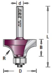
The basic edge-forming bit, the corner-rounding bit, rounds an edge to a given radius. The tool is shouldered to cut a fillet. Can be used to ease edges, as a simple profile, or as a part of a complex one.
