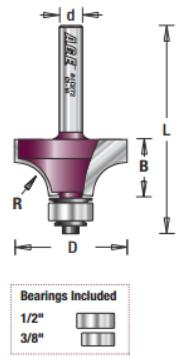
The basic edge-forming bit, the corner-rounding bit, rounds an edge to a given radius. The tool is shouldered to cut a fillet. Can be used to ease edges, as a simple profile, or as a part of a complex one.
