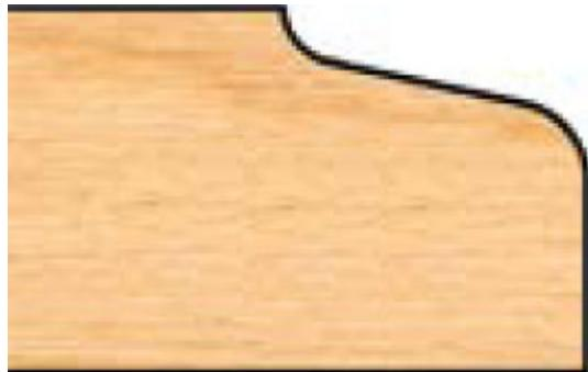
**Item #MC 57-101, Freeborn Door Edge Detail Top Cutter Only, 3/4 to 7/8" Material (32 mm Hinge System) - 3/4" Bore (Mini-Pro), 3-Wing, 2-1/16" Minor Dia**
