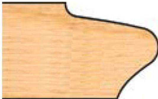
**Item #MC 57-009, Freeborn Door Edge Detail Shaper Cutter - 3/4" Bore (Mini-Pro), 3-Wing, 2-15/16" Dia, 1" Tip**
