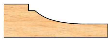
Item #MC 55-010, Freeborn Raised Panel Shaper Cutters (5/8" Material or 3/4" Material With Backcutter) 3/4" Bore Mini-Pro, 3-Wing, 4-1/2" Dia \$284.75
