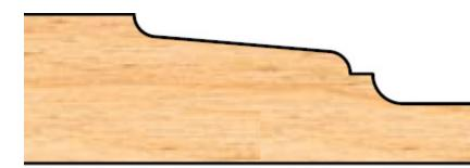
Item #MC 55-009, Freeborn Raised Panel Shaper Cutters (5/8" Material or 3/4" Material With Backcutter) 3/4" Bore Mini-Pro, 3-Wing, 4-1/2" Dia \$284.75
