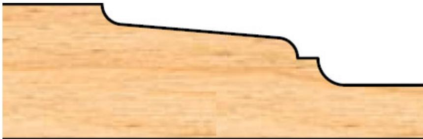
**Item #MC 55-009, Freeborn Raised Panel Shaper Cutter (5/8" Material or 3/4" Material With Backcutter)
