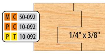
Item #MC 50-092, Freeborn (6-Piece Cutter Set) Cope and Pattern Cutter Set - 3/4" Bore (Mini-Pro), 3-Wing, 2-15/16" Dia
