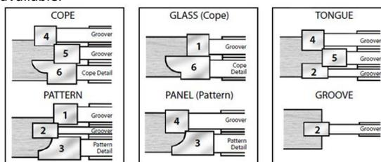
Each function of the 6 piece cope & pattern set requires a different cutter configuration. For desired results, use the following guide to set up each operation.
