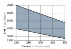
Minimum and maximum RPM based on the blade
