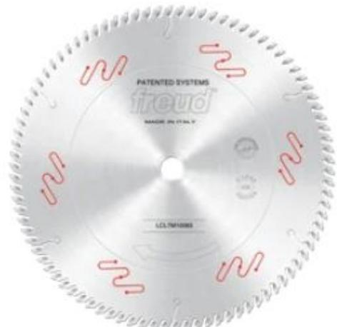
**Item #LCL7M10063, Freud Industrial 14 in Dia, 1 in Arbor, PYR+RKR, 12 deg Panel Sizing Blade (for Plywood, Particle Board, MDF Materials)**
