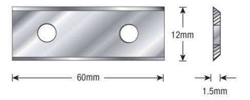
Item #ICK-60, Amana Tool Straight Solid Carbide Insert Knives: 2 Cutting Edges (Industrial) \$13.42
