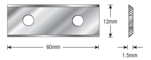
Item #ICK-60, Amana Tool Straight Solid Carbide Insert Knives: 2 Cutting Edges (Industrial) \$12.20
