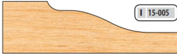
**Item #IC-15-005, Freeborn Dedicated Raised Panel Insert Cutters: 5/8" Material or 3/4" Material With Backcutter, 6 in Dia, 1-1/4" Bore**
