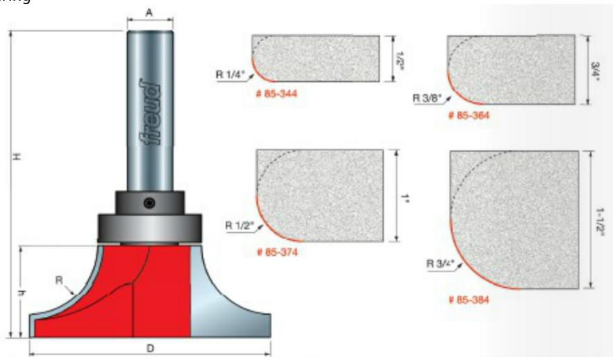
A full bull nose profile can be created by using the above the Under Rounding Bit to create the bottom round over profile and use the Rounding Over Bit (next page) to create the top round over profile.
