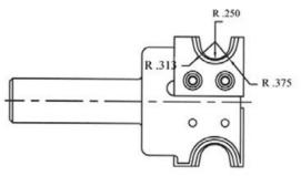
Body 8230 for material thickness of 1/2" to 3/4"
