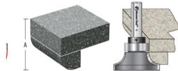
Round the lower edge of a counter with the router resting on the upper surface. No need to turn over the heavy material. This tool is especially useful for "job-site" work. (To complete a full 180° bullnose on 1/2", 1", 1 1/2", or 2" thick stock, use the corner rounding bit with the radius bearing.) Furnished with Ultra-Glide™ non-marring Delrin®-sleeved ball bearing guide.
