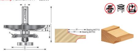
Note: Reveal ('A') reflects the total length of cut. Therefore, you must deduct 3/8" (usually) for allowing the panel to recess into the frame. Note: To receive ('A1') use bearing #47763.
