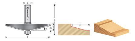
\*Reveal 'A' reflects the total length of cut. Therefore, you must deduct 3/8" (usually) to allow the panel to recess into the frame.
