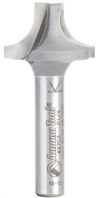
Thank you for shopping with us! This bit creates a flat-bottom groove between two quarter-round shapes. Short vertical walls extending below the radius lend extra depth to the appearance. Depending on the cut depth adjustment, the radii can be flush with the work surface, an edge guide, or on the router table using a fence.
