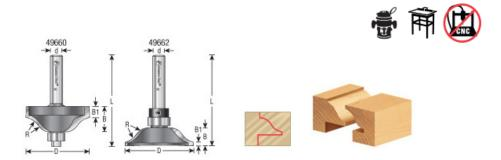
Replacement bearing for stile cutters: #47702 (3/8" dia) Replacement bearing for rail cutters: #47701 (1/2" dia) Replacement collar for rail cutters #47725
