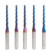
Item #46284-K-5, Amana Tool 5-Pack CNC 2D and 3D Carving 1 Deg Tapered Angle Ball Tip x 1/8 Dia x 1/16 Radius x 1-1/2 x 1/4 Shank x 3 Inch Long x 3 Flute Solid Carbide Upcut Spiral Spektra™ Extreme Tool Life Coated Router Bit \$375.49
