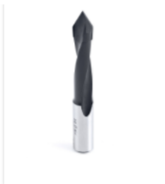
314090 Carbide Tipped Through-Hole Boring Bit R/H 9mm Dia x 70mm Long x 10mm Shank
