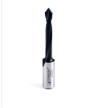
314006 Carbide Tipped Through-Hole Boring Bit R/H 6mm Dia x 70mm Long x 10mm Shank
