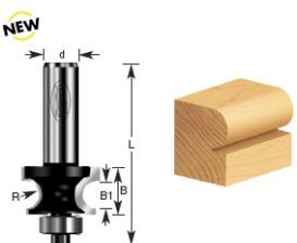
Produce three slightly different profiles using this bit—an edge bead with or without a fillet and a full corner bead—by altering the bit extension or rolling the work-piece between passes. This group of hard-to-find tools is particularly suitable for antique reproductions and restoration projects. Use in a handheld or table-mounted router.
