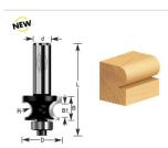
Produce three slightly different profiles using this bit—an edge bead with or without a fillet and a full corner bead—by altering the bit extension or rolling the work-piece between passes. This group of hard-to-find tools is particularly suitable for antique reproductions and restoration projects. Use in a handheld or table-mounted router.
