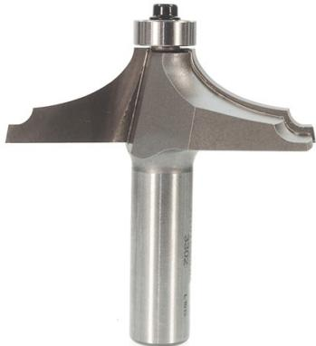
Thank you for shopping with us! Whiteside Thumbnail & Bead 1" Profile Width, 2-1/2" Lg Dia, 1/2" Shank Table Edge Router Bit has an overall design similar to a standard edge profile bit. However, the profile width is much larger for trimming the edges of a large workpiece such as a table.
