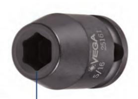
The corners of our hex and square openings have a radius for stress relief providing more torque while reducing fastener rounding
