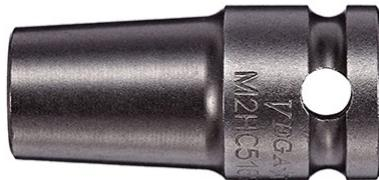
Made from high grade alloy steel. C-ring locks around corresponding grooves in bit to hold it firmly in place. Rounded corners on hex and square opening for stress relief.
