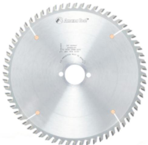
**Item #220T641, Amana Tool Carbide-Tipped Laminate and MDF 220mm Dia x 64T TCG, 10 Deg, 30mm Bore - For Holtz-Her® 220mm Panel Saws**
