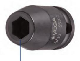
The corners of our hex and square openings have a radius for stress relief providing more torque while reducing fastener rounding
