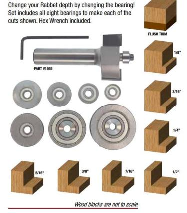
SPECIFICATIONSManufacturerWhiteside MachineCut Height, Length, or Width1/2 inLarge Diameter1-3/8 inRPM13,000-15,000 (max 18,000)
