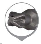
Diamond grit is embedded in the steel substrate and improves screw engagement reducing the risk of damage to the screw recess or camout. This extra hard diamond coating wears less and grips better than a Titanium coating.
