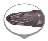
ACR\* stands for Anti-Camout Recess. The ribs on the bit tip engage the fastener recess to reduce stripping, provide increased torque, enhance off-angle drivability, and offer a stick fit that makes screw driving easier.
