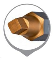
Titanium Nitride bits have a rough surface creating millions of micro gripping points. The Titanium coating provides an extra hard surface over the gripping points to protect them during use. The increase in roughness grips the entire recess of the screw and reduces camout.
