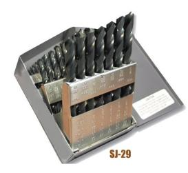
Item #06103 (SJ-29), Viking Drill & Tool General Purpose V-Line Black Oxide 118º Point HSS Drills 29-Pc Set Type 248: 1/16 -1/2" by 64ths \$88.00
