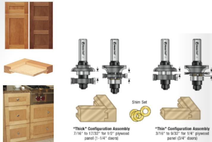
Image Right: "Thick" Configuration Assembly (7/16 to 17/32" for 1/2" plywood panel - 1 1/4" doors) Image Left: "Thin" Configuration Assembly (3/16" to 9/32" for 1/4" plywood panel - 3/4" doors) Includes full color instruction manual.
