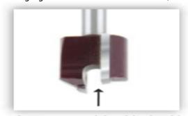
A proper mortising bit should have a large gullet between the two flutes which allows for greater chip clearance and removal.
