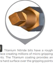
surface creating millions of micro gripping points. The Titanium coating provides an extra hard surface over the gripping points to protect them during use. The increase in roughness grips the entire recess of the screw and reduces camout.
